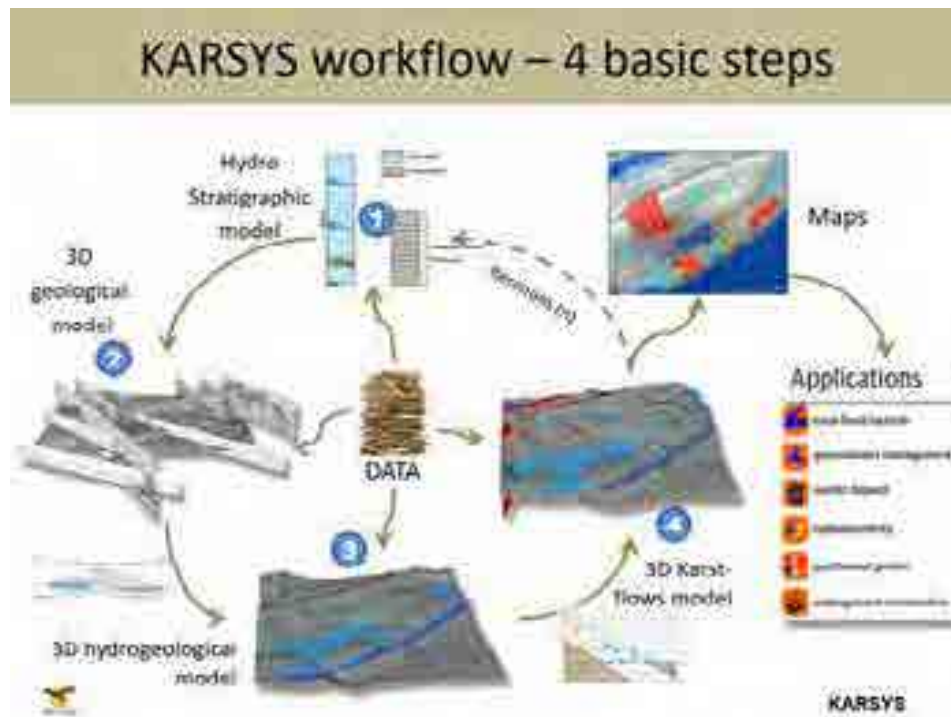
Figure 2.12: Schematic diagramme of the VisualKARSYS workflow (from end-user course held by Arnaud Malard of SISKa (Malard and Jeannin, 2022)).
